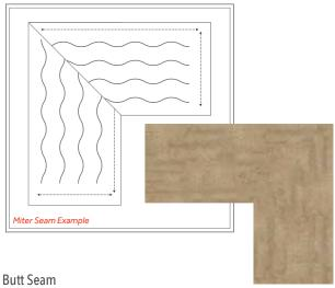
A butt seam is useful for short L-shaped counters by seaming the 30" width of the sheet to maintain a uniform directional pattern. At the seam there will be a break in the pattern which will be more noticeable with dramatic patterns. Additional 30" wide pieces can be seamed to maintain the directional pattern although each butt seam may be visible. Dry fitting the sheets and trimming material as needed to best match and orient the veining pattern is recommended.
